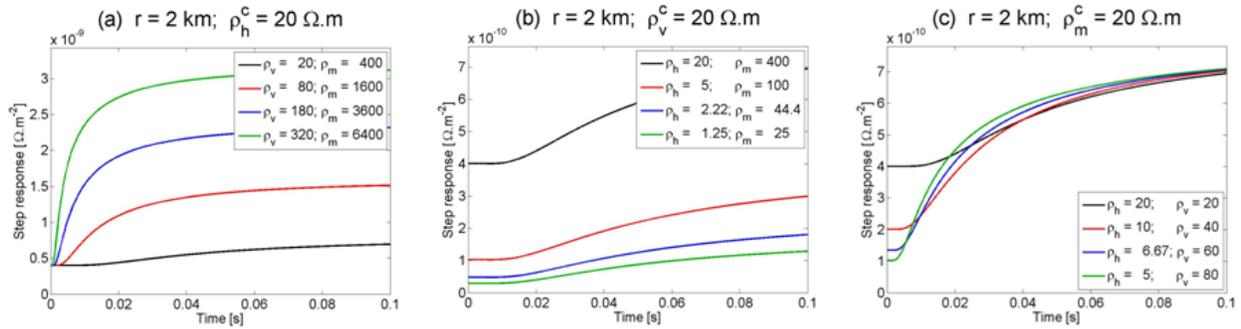
Figure 2. Effects of anisotropy on step responses at an offset of 2 km for a uniform halfspace.  $\lambda=1$  (black),  $\lambda=2$  (red),  $\lambda=3$  (blue) and  $\lambda=4$  (green). The isotropic case (solid black) is the same in all three cases.
