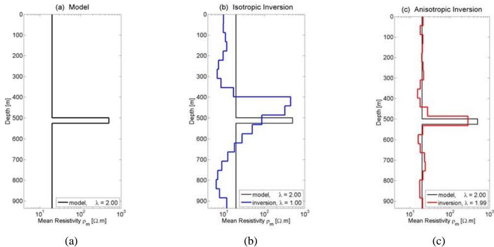
Figure 5. (a) Background resistivity model with parameters described in the text, (b) resulting resistivity model using multi-trace isotropic inversion, and (c) resulting resistivity model using multi-trace anisotropic inversion with a fixed value of anisotropy.
