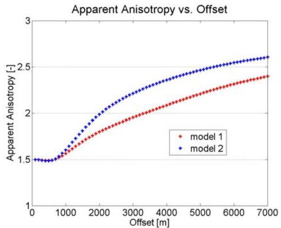
Figure 4. The apparent anisotropy defined by Equation (4) as a function of offset for the two models shown in Figure 3.
