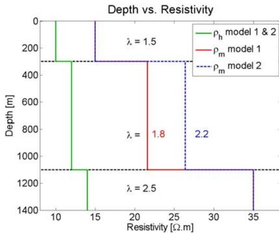
Figure 3. Two anisotropic 3-layer resistivity models. The horizontal resistivity is shown in green. The first and third layers are the same for the two models – the middle layer has an isotropy ratio of either 1.8 (red) or 2.2 (dotted blue).
