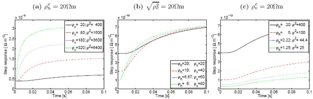
Figure 2. Effects of anisotropy on step responses at an offset of 2 km for a uniform halfspace.  $\lambda=1$  (solid black),  $\lambda=2$  (dash-dotted red),  $\lambda=3$  (dotted blue) and  $\lambda=4$  (dashed green). The isotropic case (solid black) is the same in all three cases.
