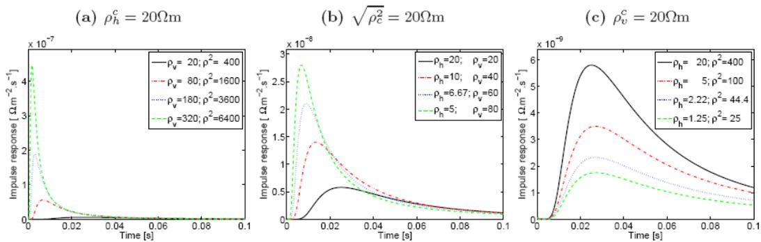
Figure 3. Effects of anisotropy on impulse responses at an offset of 2 km for a uniform halfspace (land case).  $\lambda=1$  (solid black), 2 (dash-dotted red), 3 (dotted blue) and 4 (dashed green). The isotropic case (solid black) is the same in all three cases.
